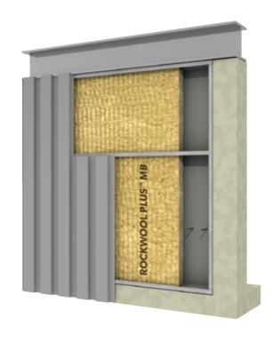
Components: Exterior Metal Cladding, ROCKWOOL PLUS™ MB, Z-Bar Girts, Flashing Channels, Wall and Partition Facings/Accessories
