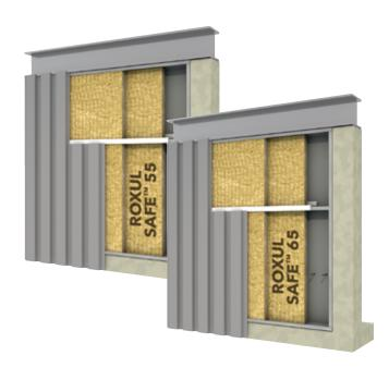
Components: Exterior Metal Cladding, ROXUL SAFE™ 55 or 65, Z-Bar Girts, Ceramic Fire Blanket (Z-Girt Cover), Flashing Channels, Wall and Partition Facings/Accessories
