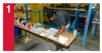
Prior to production of any faced metal building insulation order, we identify the type of facing requested and consult a chart to determine the amount of adhesive required to pass UL723.
