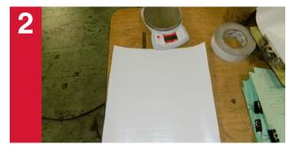
Then, we cut a swatch of the facing, weigh it, introduce it into our production process, and allow the adhesive to be applied.
