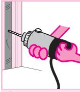
4 In the centre of the steel channel, choose one of the pre-punched holes and drill your first pilot hole for the self-tapping fastener. (Ensure at least I" penetration into the masonry.)
