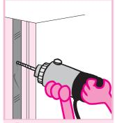
6 Repeat drilling and fastening at floor and ceiling levels. (Use a minimum of three fasteners per metal channel.)
