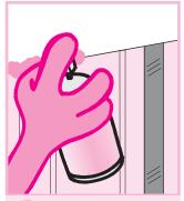
10 Fill in joint at the perimeter of the insulated wall as well as all perforations made in the insulating panel (i.e.: electrical boxes, windows) using foam sealant.
