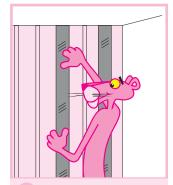
8 Insert the metal channel into the grooves along the edges of the two boards where they touch. Repeat fastening procedure, steps 4 to 7.
