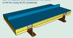
Assemblies tested in accordance with ASTM E 90. STC rating determined in accordance with ASTM E 413. OITC ratings determined in accordance with ASTM E 1332. Roof Construction is 24 ga. standing seam roof with 8" Z purlins on 5' centers. Wall Construction is 26 ga. wall panels screwed to 8" Z purlins on 7' centers.
