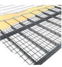
slide out from main frames and drop into position. *No fasteners or tools required, all work is done from the topside.*
