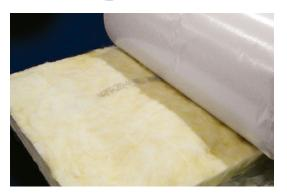
**Bay Insulation Systems' Faced Metal Building Insulation** is comprised of a resilient, light density fiberglass blanket, being NAIMA 202-96® (Rev. 2000) Insulation only, laminated to a high quality vapor retarder facing, and is compliant with the NIA Certified Faced Insulation® Standard.
