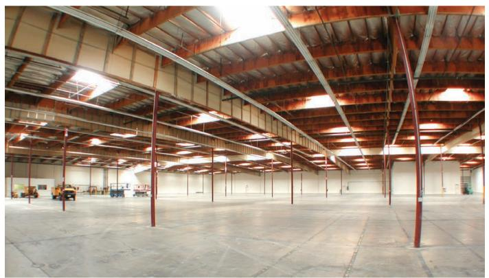
Here's the completed job. Lights are off, the hot spots are gone, and the space looks alive. Footcandles will average 79 instead of 30. At only \$0.10 per kwh, the owner will save approximately \$14,000.00 per year with a payback for this install in less than 3 years of pure after tax profit back to the company. Zero light energy also produces zero carbon emission. There isn't a more cost effective or energy efficient, green energy technology on the market today.
