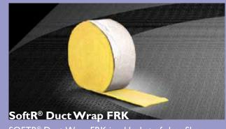
SOFTR® Duct Wrap FRK is a blanket of glass fiber insulation laminated to FRK vapor retarder facing. A 2" (50mm) stapling and taping flange is provided on one edge. It is installed on the exterior of metal duct work.
